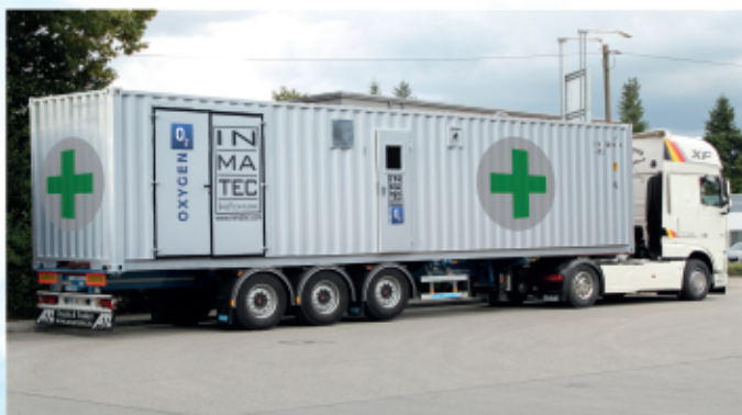
PLANT INSIDE AN ISO CONTAINER
